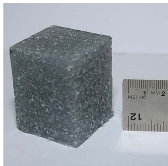
Fig. 1 The as-fabricated aluminum foam–polymer hybrid specimen
